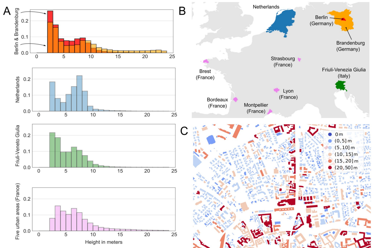
Fig 1. Building heights in the different geographical areas used in this study. (A) Height distributions for the state of Brandenburg in Germany, the Netherlands, the region of Friuli-Venezia Giulia in Italy and five French urban areas. These distributions correspond to the final dataset, after removing buildings with a height below 2 m and buildings with a footprint area below 10 m 2 , see S4 Appendix. (B) Location of the four areas representing Northern and Southern European regions, and urban and rural contexts. (C) Example of building heights in the city of Udine in Italy. This map shows a mid-size city with higher buildings in the historical center and along a main axis, and lower buildings in residential areas.
