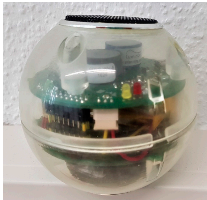
Figure 3. Schematic of the respiration measuring sphere (RMS88).
