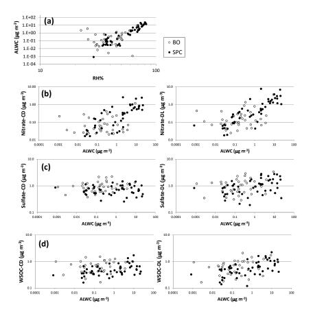
**Figure 8.** Relationship between ALWC and RH % (**a**); relationship between nitrate (**b**), sulfate (**c**) and WSOC (**d**) in the condensation (CD, left panel) and in the droplet (DL, right panel) mode of particles and ALWC averaged over the sampling periods of the Berner impactors.
