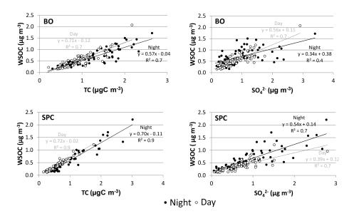
**Figure 9.** Linear regressions between WSOC and TC (left) and WSOC and  $SO_4^{2-}$  (right) in the size intervals: (1) 0.05–0.14 µm, (2) 0.14–0.42 µm and (3) 0.42–1.2 µm in daytime and at night for BO (top) and SPC (bottom).
