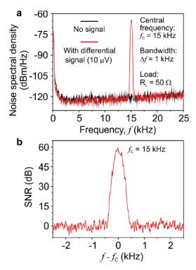
**Figure 4.** a) Noise floor of the readout circuitry circuit (-124 dBm Hz<sup>-1</sup>) measured at the output of the power amplifier without (black) and with (red) a small differential sinusoidal signal (10  $\mu$ V peak-to-peak voltage and frequency of 15 kHz) applied at the input of the operational amplifier. Bandwidth is 1 kHz. The GMR bridge is not connected. b) Magnified spectral density demonstrating the SNR of 56 dB.
