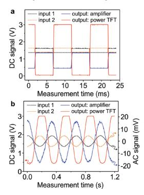
**Figure 3.** Intermediate response of the operational amplifier (blue) and overall output of the readout electronics (red) on an externally applied square wave (a) and sinusoidal (b) differential input signals. The data reveal a total open loop gain of 48.6 dB, whereas the supply voltage was 3 V and the oscilloscope (1 M $\Omega$ ) was used as a load element.
