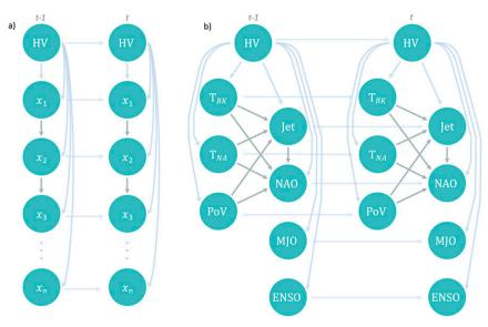
FIG. 3. Example DAGs. (a) A DBN with a single hidden variable unrolled over two time slices with autoregressive links between all variables. Gray arcs in the "intra" (within a time slice) graph represent links between observed variables, with autoregressive links shown in the "inter" (between time slices) arcs. (b) As in (a), but for a summarized graph of the 5-day jet HV DBN used in this study.
