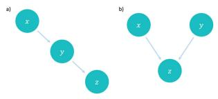
FIG. 2. Example DAGs: (a) x and z are conditionally independent given y therefore no arc between x and z is needed or parameterized, and (b) an example of a collider structure, where node z has two parent nodes, x and y.
