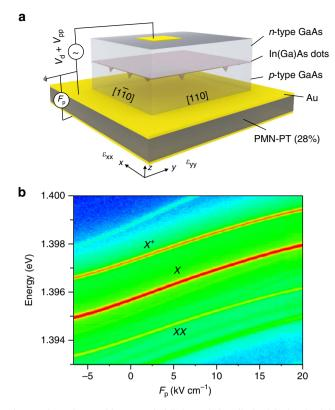
**Figure 1 | Strain-tunable entangled-light-emitting diode. (a)** Sketch of the diode structure. Different from previous works, the PMN-PT top surface has (011) orientation, which imposes large anisotropic strain fields with well-defined orientation onto the overlying ELED. (b) EL from a single QD in an ST-ELED versus electric field  $F_p$  applied to the PMN-PT actuator.
