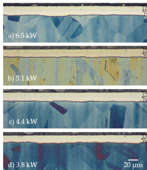
Figure 4. Resulting duplex layer formation for (a) 6.5 kW, (b) 5.1 kW, (c) 4.4 kW, and (d) 3.8 kW using a gas composition of N_2:H_2 = 1:1 ; T = 733 K; t = 5 h; etchant: Beraha II reagent.
