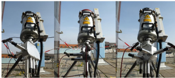
Figure 1 POLIS-6 with the receiving optics rotated at \pm 45^\circ (left, right) for the \Delta 90^\circ -calibration, and at 0^\circ (middle) for atmospheric measurements.
