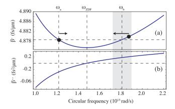
Figure 1: A typical profile of (a) the group delay  $\beta'(\omega)$  and (b) group velocity dispersion  $\beta''(\omega)$  that leads to the collision phenomenon shown in Fig. 2. Collision can only be realized for initial DW frequency offsets in a small interval (shaded grey) around the reference frequency of matching group velocity.
