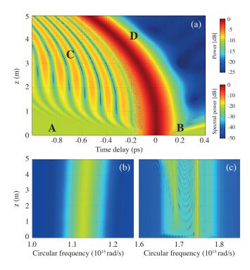
Figure 2: An exemplary reflection of a DW from a soliton. (a) Normalized power in space-time representation. The DW is less intense than the soliton. The chosen frame of reference copropagates with the unperturbed soliton. (b,c) normalized power in frequency domain for soliton and DW respectively. See Fig. 1 for the carrier frequencies and text for explanation of the patterns A–D.
