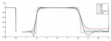
**Fig. 16** The 3d example: the approximations shown in Figs. 11 (SUPG), 12 (BBK), 13 (BJK), 14 (Kuz) and 15 (reference) on the line y = z = 1
