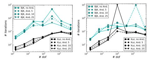
**Fig. 6** Hemker example: number of iterations for solving the nonlinear problems, for  $\omega = 0.5$ , l = 5, 10, 25 vectors in the Anderson acceleration, on Grid 1 (left), Grid 2 (right); 100,000 iterations means that the stopping criterion was not reached
