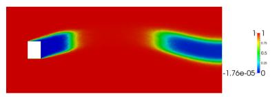
Fig. 14 The 3d example: the slice at z = 1 of the approximation obtained by the Kuzmin limiter. It took 70 iterations for the Euclidean norm of the residual in the damped fixed point algorithm to be less than the tolerance of  $10^{-6}$
