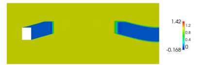
Fig. 15 The 3d example: the approximations obtained using the SUPG method on an adaptively refined mesh containing 135, 408, 953 elements
