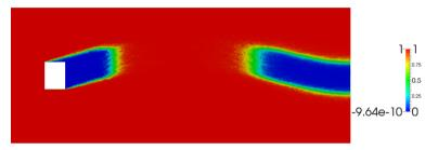
Fig. 13 The 3d example: the slice at z = 1 of the approximation obtained using the BJK method. It took 1117 iterations for the Euclidean norm of the residual in the damped fixed point algorithm to be less than the tolerance of  $10^{-6}$
