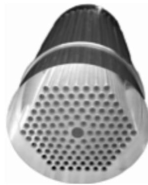
Fig. 1. Digital camera photograph of the drilled preform with a diameter of 60 mm.
