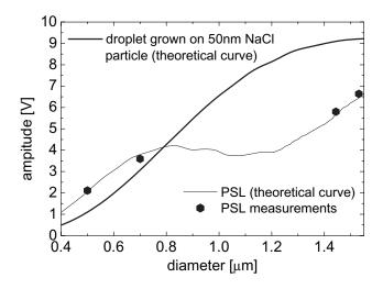
**Fig. 2.** The response curves for the conversion of the amplitudes of the signals measured with the optical particle spectrometer to droplet diameters, for PSL particles and for droplets grown on NaCl particles with a dry diameter of 50 nm.
