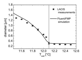
**Fig. 4.** Measured and simulated droplet diameters at the LACIS outlet for varying wall temperatures, for NaCl particles with a dry diameter of 50 nm.
