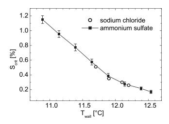
Fig. 5. LACIS calibration curve for the relation between  $T_{wall}$  and critical super-saturation.
