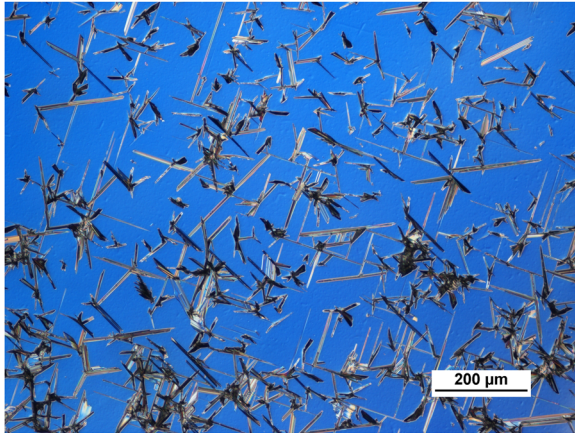
FIG. 4. ZnO overgrowth on a ZnGa 2 O 4 wafer embedded in ZnO powder during annealing in air at 1200 °C for 10 h with the mass gain of 0.47 wt. %.
