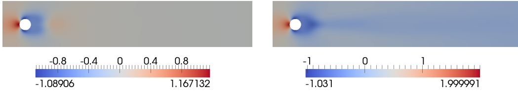
Fig. 8. High accuracy snapshots (SP-NONLIN): pressure coefficient p_{00}(\mathbf{x}) computed with VMB-ROM (left); pressure coefficient \bar{p}(\mathbf{x}) for PCM-ROM and SM-ROM (right).
