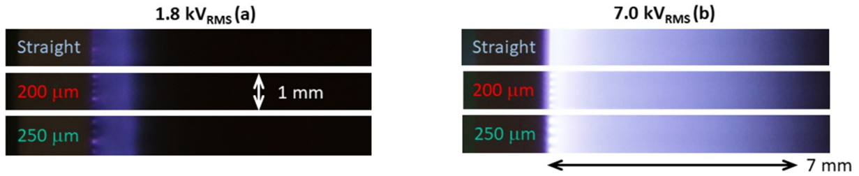
Figure 2. Top view of electrode structure photographed by Canon EOS 77D under 1.8 kV RMS (a) and 7.0 kV RMS (b) operation voltage, 0.5 mm samples.
