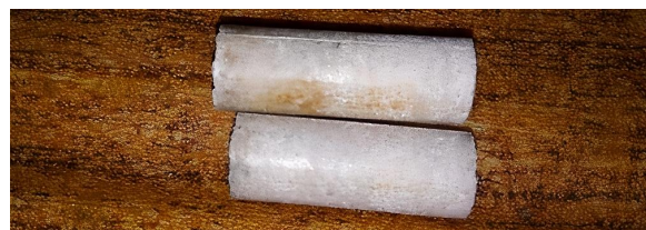
Fig. 1. Sample bone for compressive test
