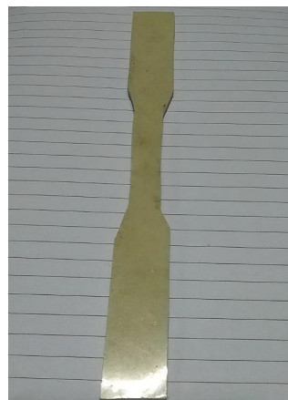
Fig. 2. Specimen for tensile test
