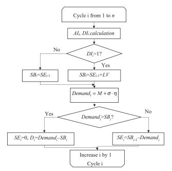
Fig. 3. Simulation algorithm with the threshold strategy
