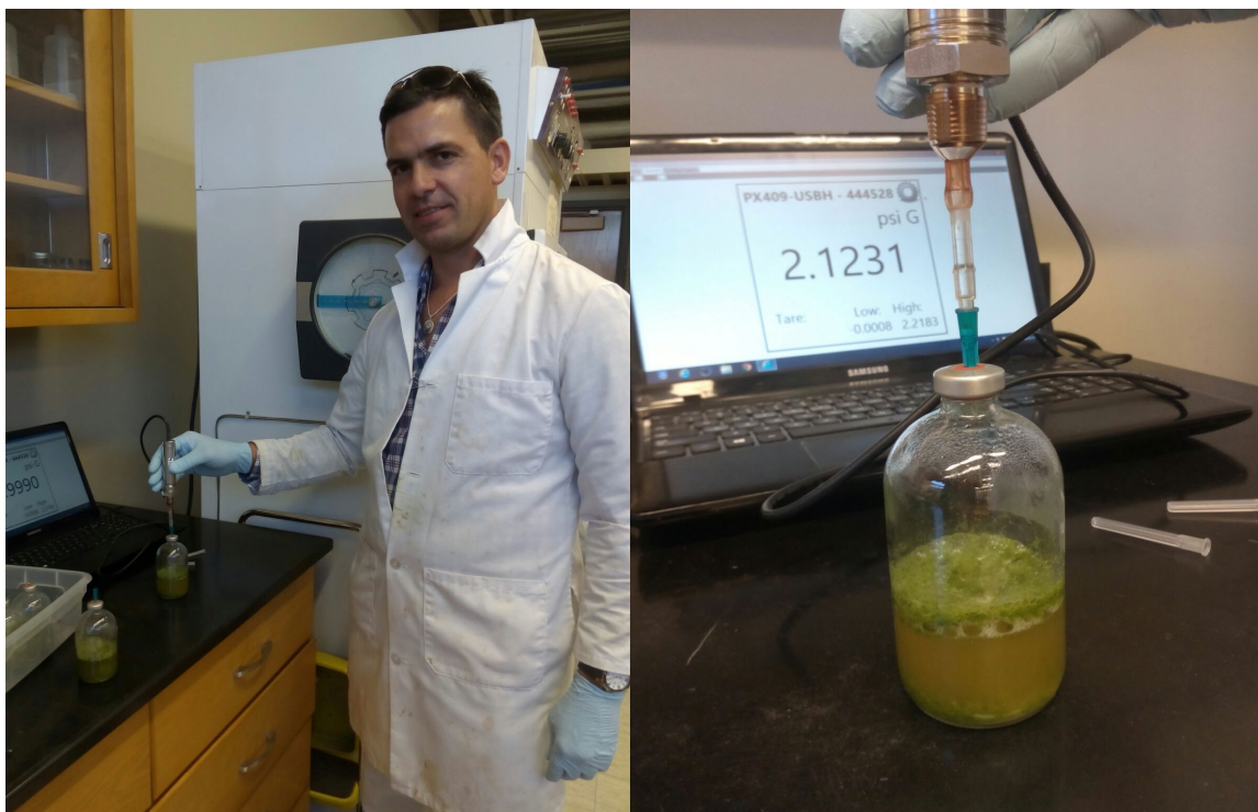
Figure A-4. Measurement of the head-space gas pressure of the flasks with an USB output pressure transducer.
