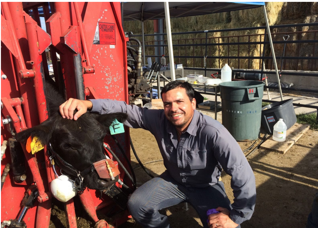
Figure A-9. Heifer fitted with a halter and evacuated canister for enteric methane collection.
