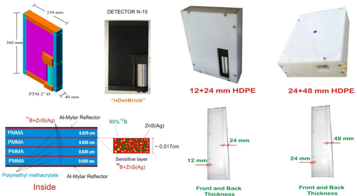
Fig. 1. Configurations of “nDetBrick” detector. Inside view section.
