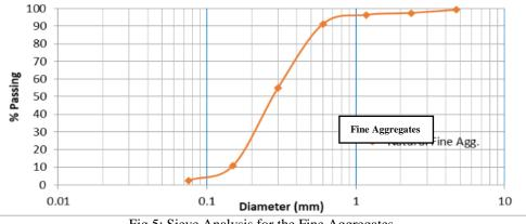
Fig.5: Sieve Analysis for the Fine Aggregates
