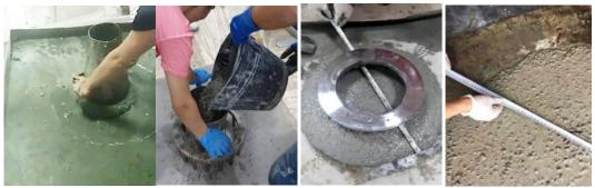
(a) (b) (c) (d) Fig.8: Slump Flow, Visual Stability Index (VSI), J-Ring, and T<sub>500</sub> Tests
