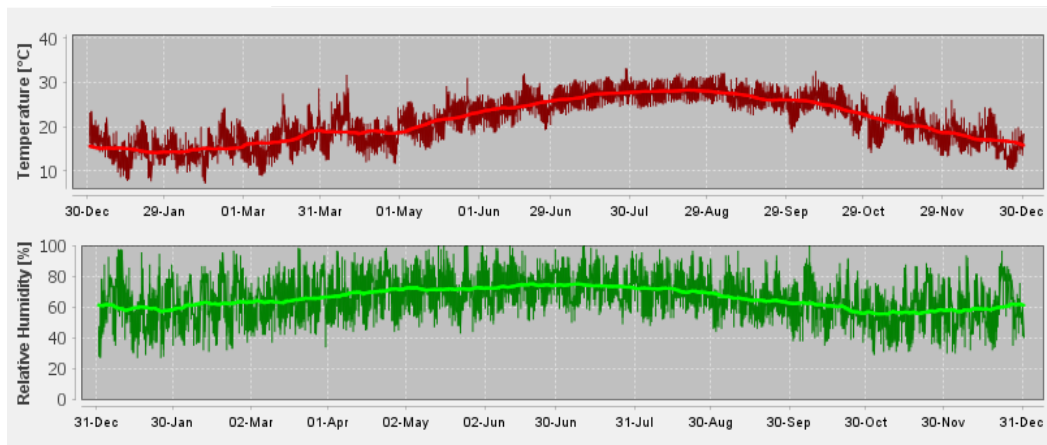
Fig.2: temperature and relative humidity data recorded for the year 2018, used in the simulation Reference: Wufi pro capture based on data file from Beirut Airport forecast station
