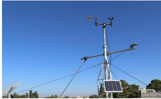
Figure (3): The meteorological station – Engineering Building
