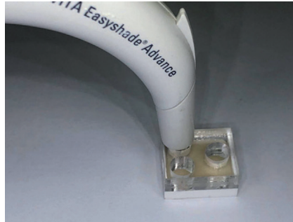
Figure 8: The spectrophotometer positioning through the access holes
