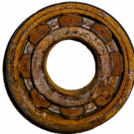
Figure 1. Ball bearing with heavy corrosion.
