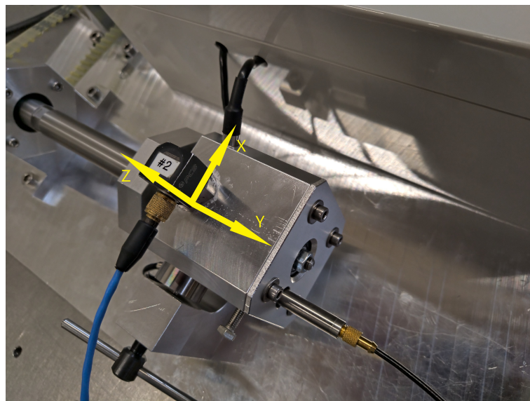
Figure 6. Coordinate system of the triaxial acceleration sensor.
