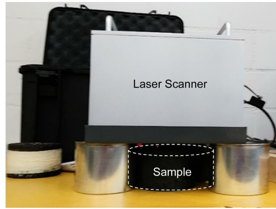
Fig. 6. Scanning asphalt texture with Ames Engineering 9400HD 3D laser scanner.
