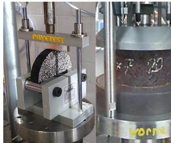
Fig. 4. Semi-circular bending (SCB) testing (left) after conditioning at 0 °C (EN 12697-44) and cyclic compression test setup [52] (right).
