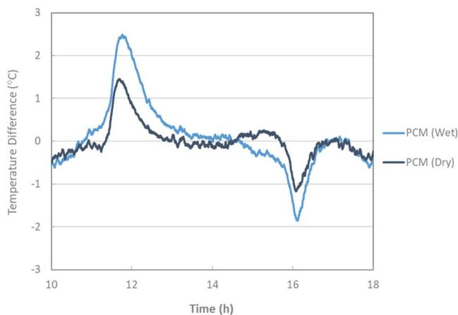
**Figure 7.** Temperature difference evolution between mixtures of PCM (dry and wet) with mineral (reference).
