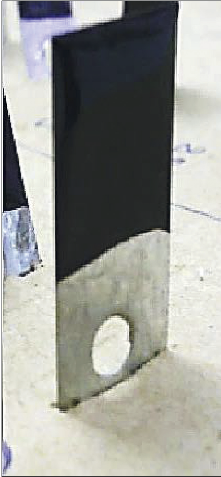
FIGURE 3: Metallic strip coated with binder.
