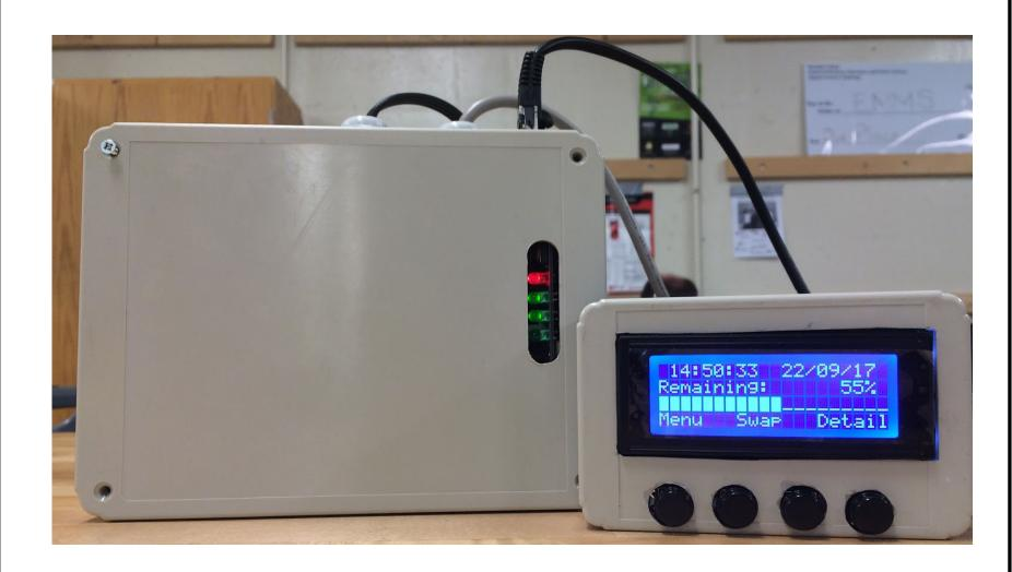
Method **Method:** Our solution consists of a meter which allocates a configurable daily energy limit per facility, along with a display that provides feedback to the user. This display includes information about how much energy remains in a day and how much power is being used at any time.
