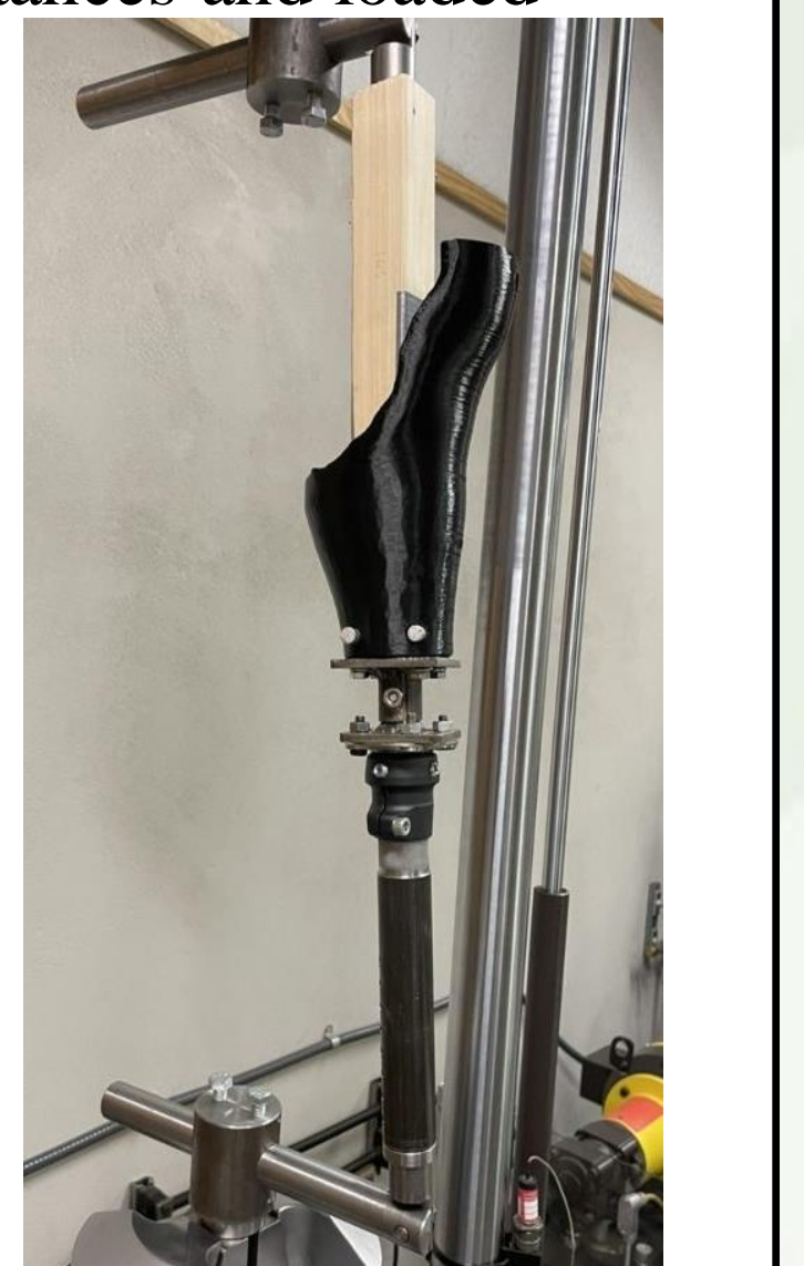
Full Assembly of Testing Rig in MTS Machine
