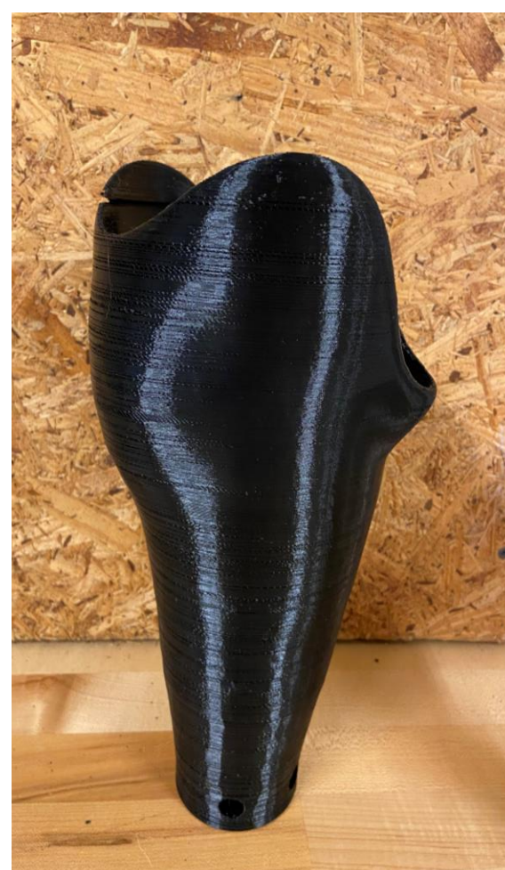
3D Printed Transtibial Socket
