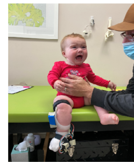
Figure 3: One of Mr. Cunningham's patients wearing the force testing system on their brace.
