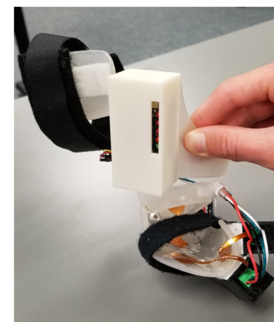
Figure 2: Cunningham brace with force testing system applied.
