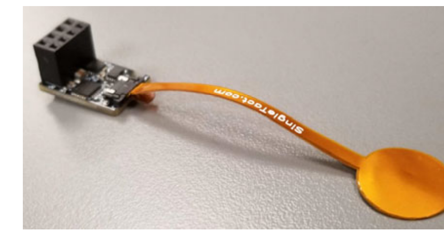
Figure 1: Capacitance force sensors used on both braces
