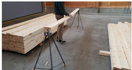
Figure 1. MOE and specific gravity measurement using Metriguard E-computer Model 340 dynamic tester.
