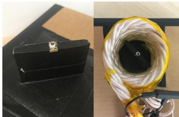
Figure 6.1 Setup for heating experiments in air. A fibre optic temperature probe was supported with a cardboard structure, allowing the tip to be pointing up vertically. The thermoseed was positioned on and in contact with the tip of the probe (left). The coil was placed around the cardboard support, with the thermoseed positioned in the centre of the coil to align within the maximum field generated by the coil.
