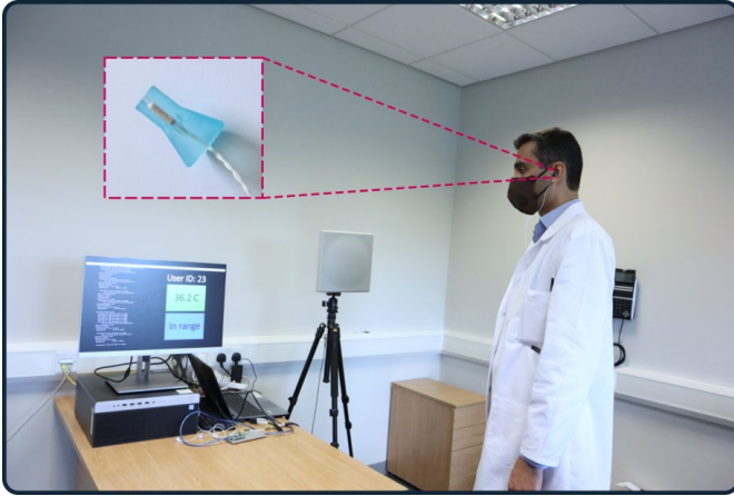
Figure 3: System setup showing sensing system, reader, antennas, and test setup
