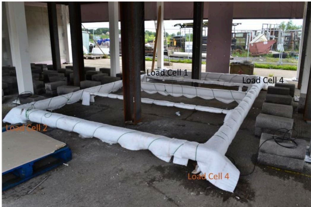
200 Figure 4: Mass load recording frame with load cells and fire protection arrangements of the steel frame used for mass loss 201 recording
