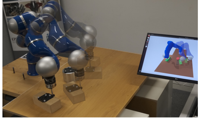
Fig. 1. Experimental setup where the robot plans and controls the motion of an object to push it to the target, via sliding contact and while avoiding an obstacle.
