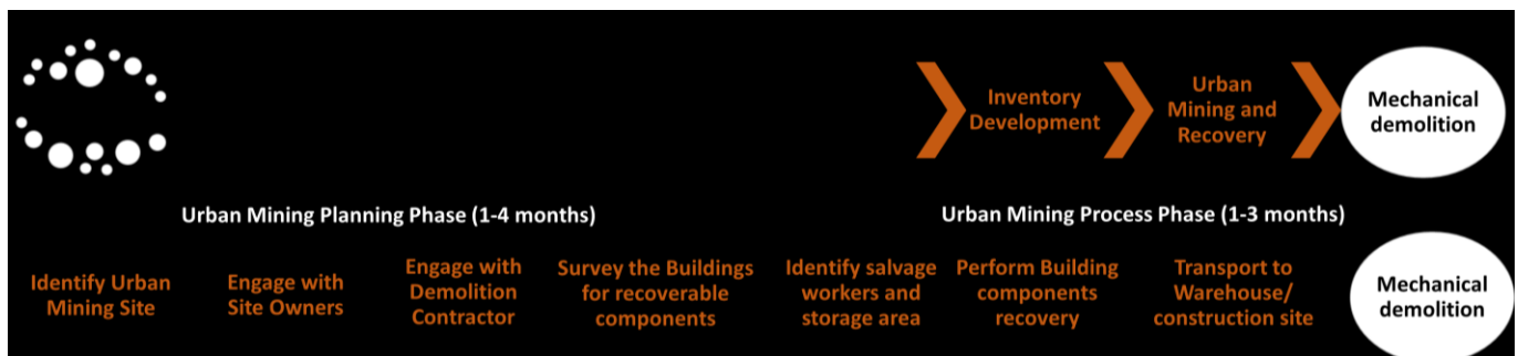
352 Figure 3. Inclusion of urban mining planning and process into the demolition project strategy
