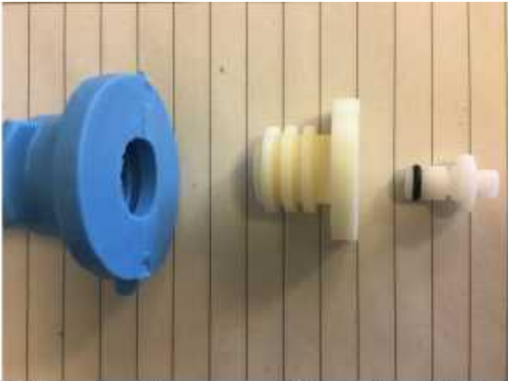
Fig. 3. Finger opening, plug and fitting (from left to right)
