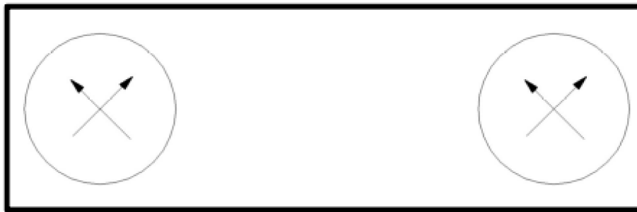
Figure 11. RSR beams are separated on the sky by \sim 78'' ( \sim 5 times HPBW). At any given instant, as the 1 kHz beam switch changes sign, the two orthogonal polarizations in each beam are received by four independent pixels.
