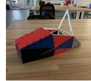
3D printed implementation of car shelling. Future plans to scale up and laser cut wood.
