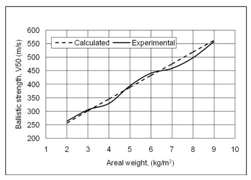
Figure 1. Ballistic strength vs. areal weight of composites
