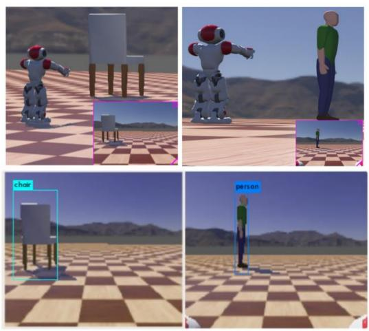
Figure 5. Top: NAO interacting in the virtual environment. Bottom: chair and person detection on embedded systems. Source: Created by the authors.
