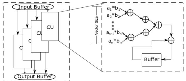
Figure 2. Hardware architecture of the PipeCNN framework. Source: Created by the authors.
