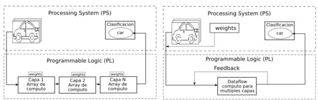
**Figure 3.** Types of FINN framework architectures: (a) DF architecture with defined layers and weights. (b) MO architecture with layers and weights for different accuracies and sizes. Source: Created by the authors.
