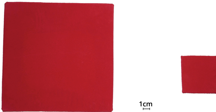
Figure 4.8.: Reflectors used in the spacer study: large reflector ( 15\text{ cm} \times 15\text{ cm} , left) for the reference measurement and small reflector ( 5\text{ cm} \times 5\text{ cm} , right) for the spacer measurements.
