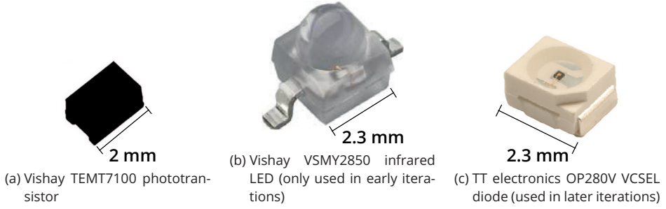
Figure 4.5.: Optical components for the distance sensors. The VSMY2850 LED was replaced by the OP280V vertical-cavity surface-emitting laser (VCSEL) diode in the later iterations of the EOS system.
