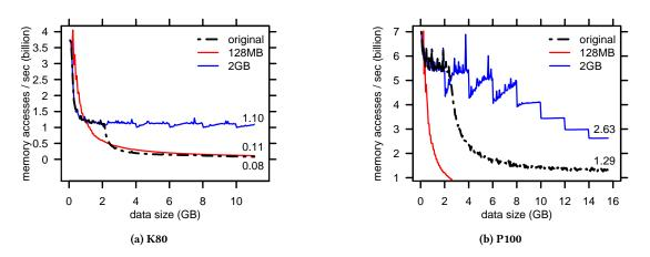
Figure 10: Random sampling with different TLB scope sizes.
