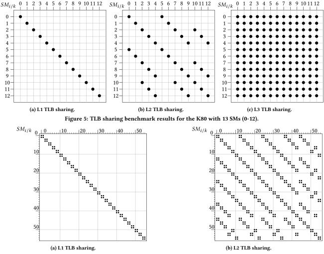
Figure 6: TLB sharing benchmark results for the P100 with 56 SMs (0-55).
