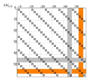
Figure 12: Hypothetical L2 TLB sharing with 60 SMs (0-59). Four SMs were added (gray) and four SMs were swapped (orange).
