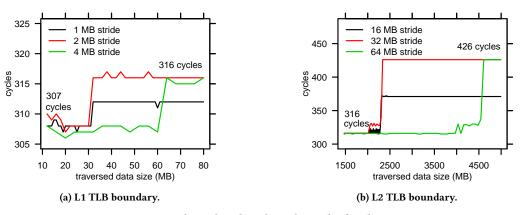
Figure 4: TLB boundary benchmark results for the P100.
