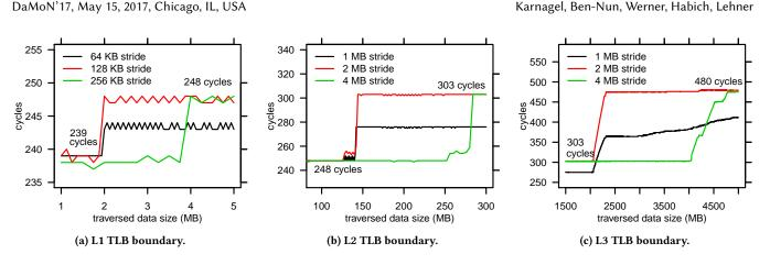
Figure 3: TLB boundary benchmark results for the K80.
