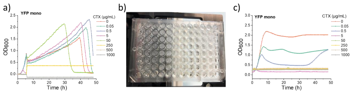
Figure 69: OD 600 of monoculture E. coli YFP incubated and measured in transparent microplates in various CTX with and without membrane, a) growth curves monitored with membrane, b) transparent microplate attached with membrane and c) growth curves monitored without membrane.
