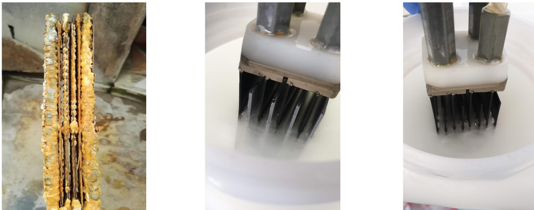
Fig. 23a-c: Completely clogged electrolytic cell during pilot trial in WB India [P1.3] and new setting as tested during pilot trial in Almeria Spain [P3.3] with extremely hard waters
