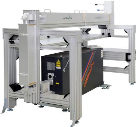
Fig. 3-3. Basic scheme of a FLA tool used for semiconductor wafer processing. From ref. [101].
