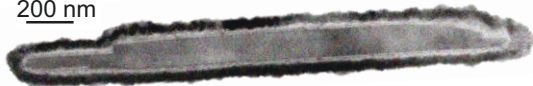
Figure 1: TEM image of Iriotec®7550 particle in cross section, with mica core and doped tin oxide shell.
