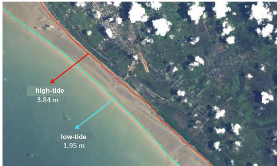
Figure 16. Intertidal zone from imageries of different tidal conditions (Amhar & Subagio, 2012)
