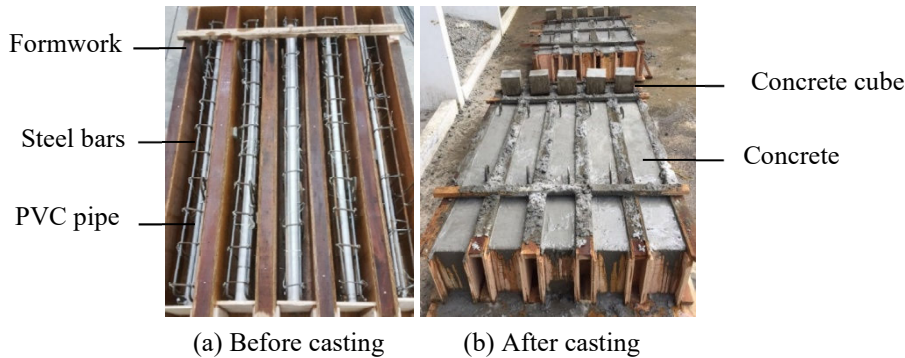
Fig. 4. Fabrication of beam specimens.
