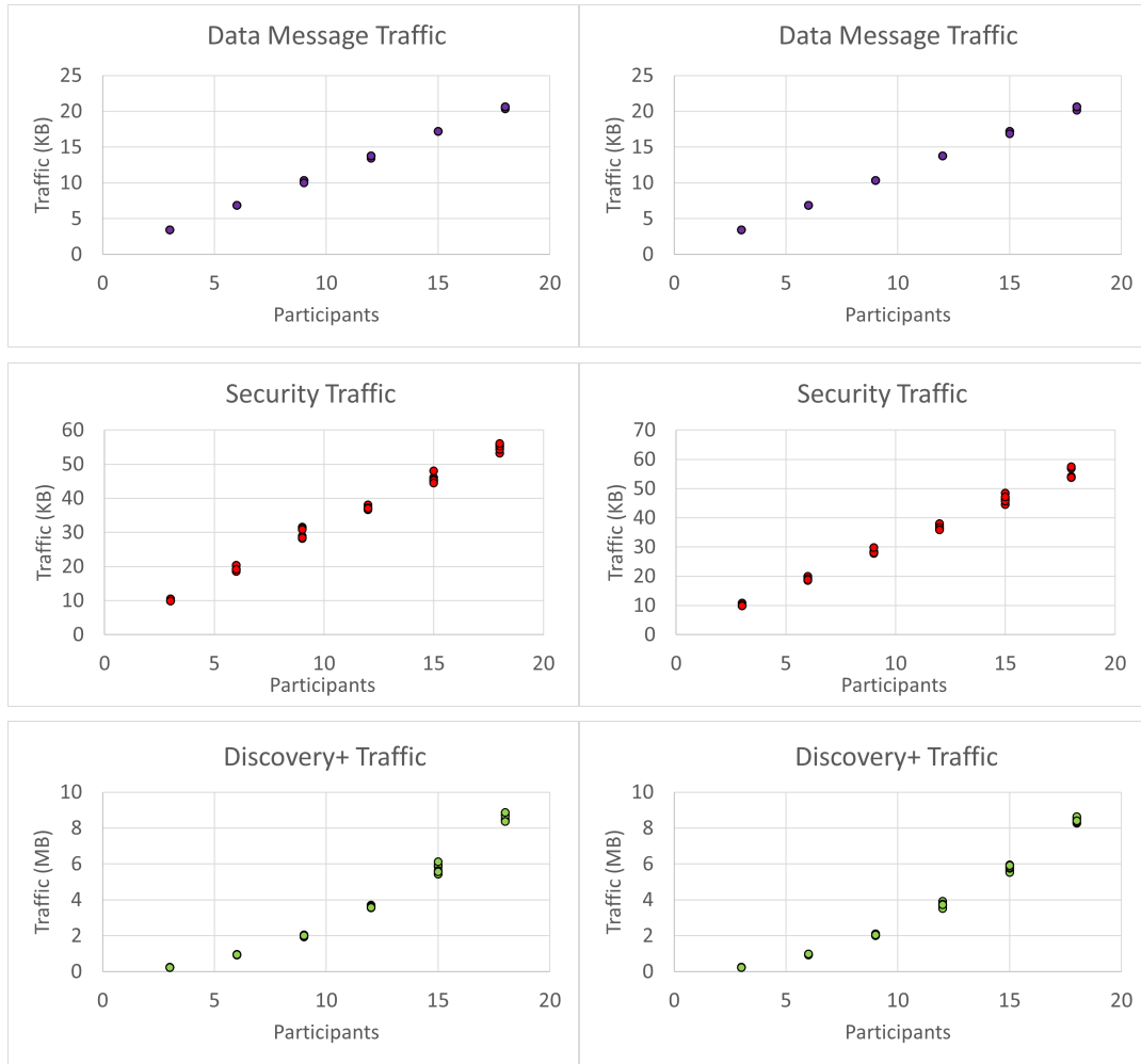
Fig. 8 Experiment Results. Left column: Best Effort Foxy1 with Kerby. Right column: Reliable Foxy1 with Kerby.
